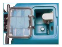
Unique tank design channels air flow to separate water from air and reduces foaming. The ball float designed prevents solution or foam from flowing into vacuum fan.
