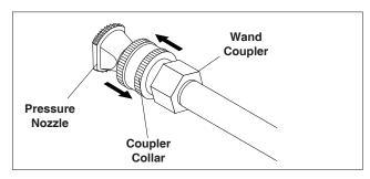
**STEP 7:** Pull the spring-loaded collar of the wand coupler back to insert your choice of pressure nozzle. Release the coupler collar and push the nozzle until the collar clicks. Pull the nozzle to make sure it is seated properly.
