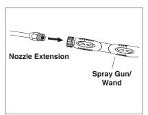
**STEP 2:** Attach nozzle extension to spray gun/wand. Tighten both by hand.
