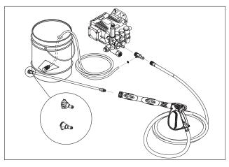
**STEP 2:** With safety latch on spray gun engaged, secure black detergent nozzle into quick coupler. **NOTE:** Detergent cannot be applied using the yellow nozzle.
