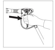
**STEP 5:** Trigger the spray gun to eliminate trapped air then wait for a steady flow of water to emerge from the spray wand. Then install nozzle.
