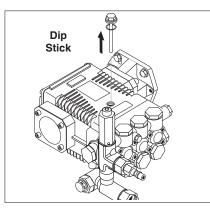
**STEP 2:** Remove shipping cap and install oil dipstick. Check pump oil level by using dipstick or observe oil level in oil window (if equipped). Use 30 wt. non detergent oil.
