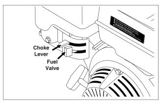
**STEP 7:** Move the choke lever to the "Choke" position (on a warm engine, leave the choke lever in the run position). On Honda engines, move the choke lever to the "Closed" position. To restart a warm engine, leave the choke lever in the "Open" position.
