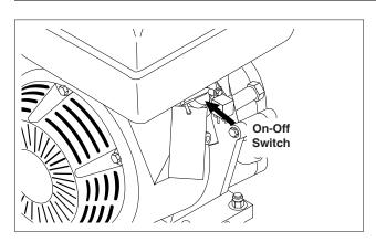
**STEP 8:** On Honda engines, turn the engine switch to "On" position.
