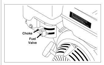
**STEP 6:** Rotate the fuel shut-off valve to the "On" position (fully counterclockwise on Briggs engines). Slide the fuel valve lever to the "ON" position (Honda engines). When the engine is not in use, leave the fuel valve in the "OFF" position.
