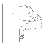
**STEP 3:** Before installing nozzle, turn on water supply and run machine allowing water to flush through the system until clear.
