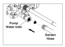
**STEP 5:** Connect the garden hose to pump water inlet. Inspect inlets. *CAUTION: Do not run the pump without water or pump damage will result.*
