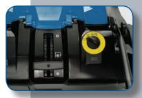
Main roller brush easily adjustable in six positions.
