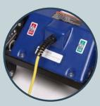
Saftey switching system prevents accidental start-ups. If cord is unplugged during use, the GROUTHOG won't start when reconnected until "on" switch is pushed.
