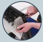
To change brushes, simply undo the forward thumbscrew, mount the new brush, and reassemble —it's done in seconds!
