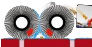
Choose the cylindrical scrub brush head for floors with occasional debris, or for tile surfaces. It simultaneously scrubs and picks up small debris.
