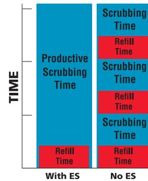
feature saves you time and improves your productivity. What's more, you can clean up to 3 hours without interruption. ES™ uses less solution and less water, effectively eliminating down time spent emptying and refilling solution and recovery tanks.
