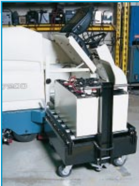
Roll-out battery package extends run-time and is easily changed in less than 5 minutes.
