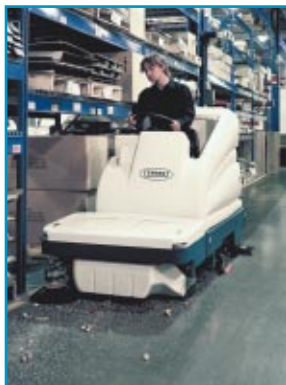
The optional sweeper attachment allows the 7200 to sweep and scrub in one pass.
