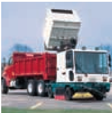
The 830-II's 9½-ft. (2.89 m) high-dump allows for discharge into large roll-offs and dump trucks.
