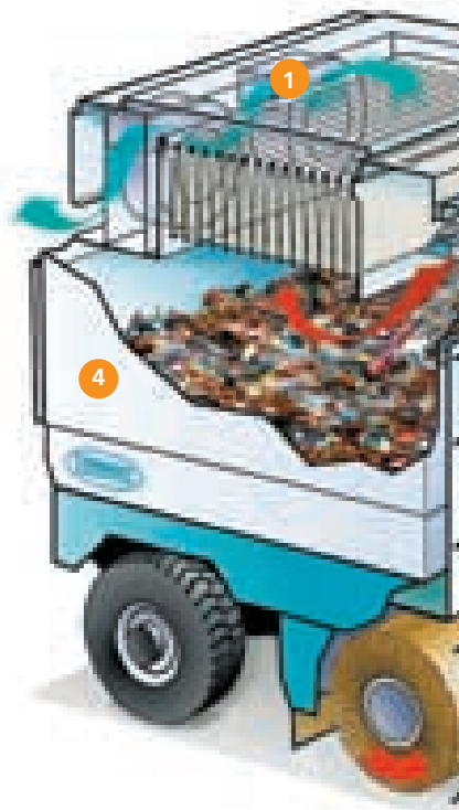
Innovative dry-dust control improves ambient air quality by sucking up dust and dirt stirred up by brushes.
