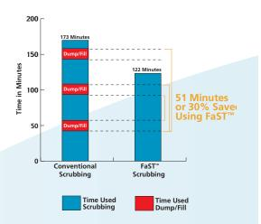
Assumption: Dump and fill time is set at 17 minutes for a 32-inch scrubber. Cleaning speed is 1.5 mph.
