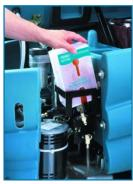
Compact, conveniently located, and easily installed, the FaST-PAK cartridge accurately meters FaST concentrate for optimum cleaning performance.
