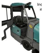
Increase safety and effective operation, in even the most severe environments, with an optional FOPS certified (ISO 3449) pressurized cabin available with heat
