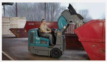
Dumps at any height from ground level to 60 in (1525 mm) and reaches up to 30 in (760 mm) into the dumpster. Contain debris during transport with a hopper equipped with a rear hopper door.
