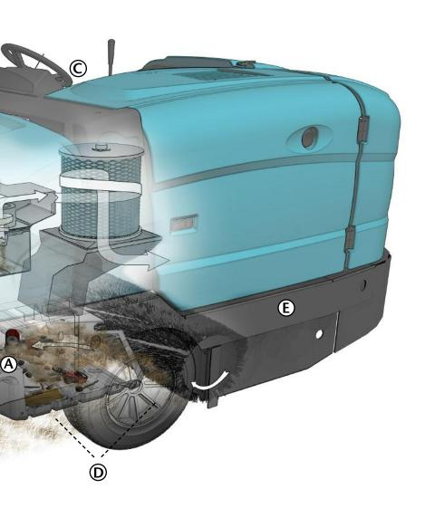
Effectively remove different types of debris with the II-Speed™ sweep system. This increases the speed of the main brush, side brush, and vacuum fan by 20%.
