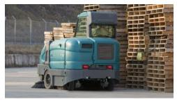
Travel between work sites safely and quickly with the S30 X4 configuration that travels up to 15 mph (24 kph) on a stable 4 wheel platform with comfortable leaf spring suspension.
