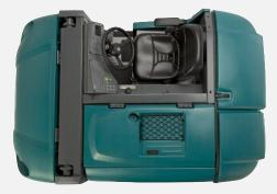
Enhance operator safety and productivity with a cab forward ErgoSpace™ operator compartment that improves operator comfort and visibility.
