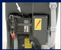
Onboard battery charger eliminates lost chargers and makes recharging easier
