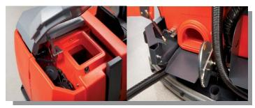
82 gallon solution and recovery tanks offer a longer cleaning time before dumping recovered water and filling with fresh water. The recovery tank offers easy access for complete clean out.
