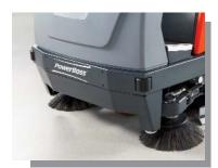
The standard sweep system allows for collection of dirt and light debris into the hopper, therefore allowing sweeping and scrubbing in one easy pass.
