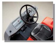
One touch operator controls. Press the green button and you are Power cleaning. The open operator compartment provides excellent visibility and entrance or exit from either side of the machine.
