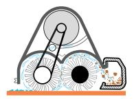
Choose disk scrubbing (above) or cylindrical scrubbing (below) with debris pick up to meet facility's cleaning needs.
