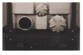
Oversized cleanout ports with simple screw-on caps facilitate recovery tank draining and sludge removal.
