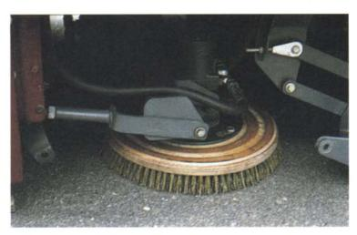
Quick-change disc scrub brushes help remove years of caked, oily dirt build-up. Scrub head floats for constant floor contact.
