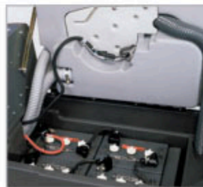
Hinged recovery tank with safety latch gives easy maintenance access. Vac motor has sound deadening for quiet operation.
