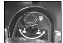
The pad-adjustment knob allows the operator to fine-tune pad pressure.
