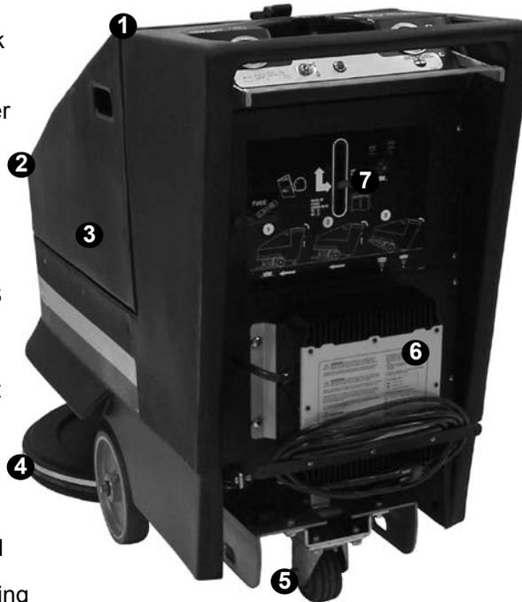
⑦ Using the tilt lever, the machine can tip from the operating to the transport to the pad change position.
