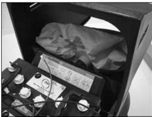
The Vac-Trac Dust Control System collects dust and deposits it in a filter bag at the front of the machine.
