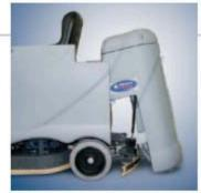
No tools are needed to lift off recovery tank for extra access to batteries and squeegee assembly.
