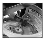
80% safety fill type propane tank. All propane system components are UL approved.
