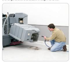
The Tip-out recovery tank makes equipment clean-up safe and simple and helps keep your recovery tank fresh.
