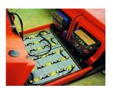
Environmentally-friendly battery drive. Quick exchange of battery trays in approx. 2 minutes with fork lift truck or lifting equipment
