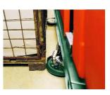
Suspended, floating side scrubbing unit (option) for working close to the edge, near walls, pallets and under shelves.
