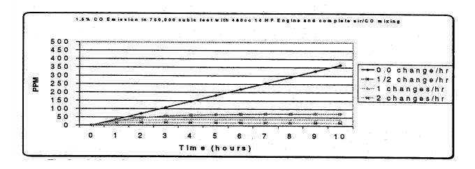
Based on the CO production rates shown above the TWA would be exceeded in a  $100 \times 500 \times 10$  foot (empty) space after 6 hours with 2 air changes per hour. (Assumes no additional CO exposure during 8 hour time period).
