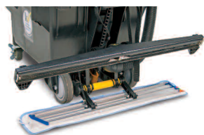
Spread Only Extended dwell time for heavy soil, disinfection, etc.
