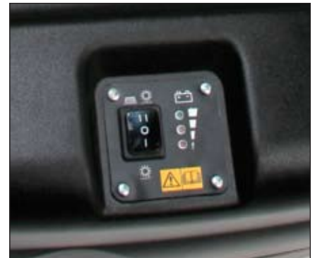
A single switch and battery level indicator allows for minimal operator training.
