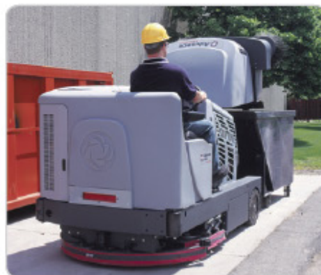
The ergonomic Clear-View™ design provides the operator with an unobstructed view of critical sweep zones
