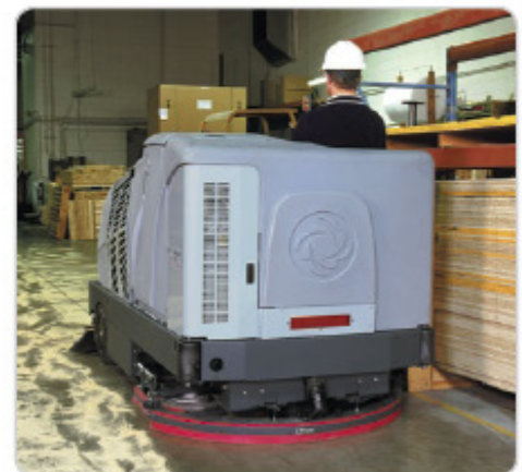
Aggressive scrub system removes ground-in dirt, while the squeegee leaves floors dry. Combined, you get complete cleaning in a single pass
