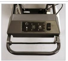
Touch Pad Controls — Controls are conveniently located. Solution control, master on/off, vacuum and brush switches are located at your fingertips.
