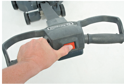
Red SafeStart™ button only operates in operator position.
