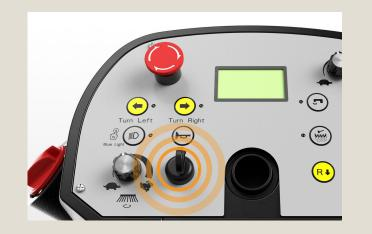
Insert the operator key, and turn to start the sweeper.
