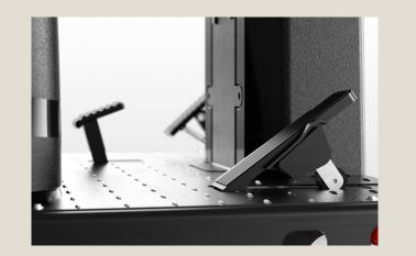
The brushes and vacuum will start when the drive pedal is pressed, start sweeping.
