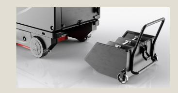
Press the OneTouch<sup>™</sup> button to stop all functions. Slowly release the hopper locking mechanism as it may be heavy. Use the handle to remove and empty the hopper.
