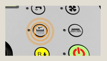
Press the filter shaker button to clean the filter. Hold the button until the light blinks to enable automatic shaking every 10 minutes.
