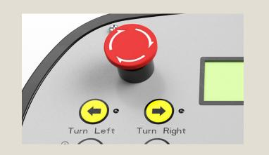
Use the turning signals when turning, right/left lights located only in the rear.
