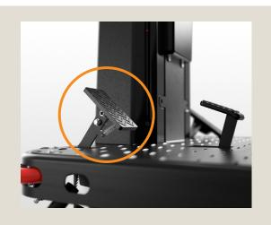
4. Check if the parking brake pedal is engaged.
