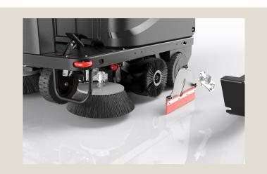
Ensure the main broom and side brooms are properly installed.
