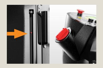
Check the solution level on the side of the machine. Add fresh water as needed by removing the red cap on the fill port.
