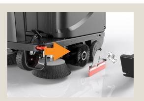
Inspect the main broom, make sure it's turning and is not worn out. Adjust broom pressure if needed.
