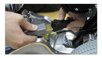
**4.** Connect the power cord from the base of the handle to the motor.
