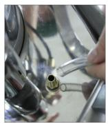
**3.** Connect the hoses for solution spray and gravity feed as shown above.
