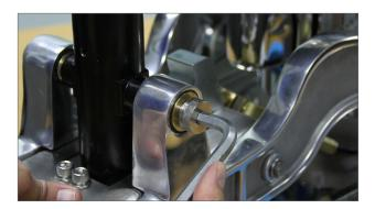
1. Set the handle assembly in place and bolt it in using the two included bolts. Thread the bolts in by hand as far as you can in order to prevent stripping of the threads in the handle. Tighten with 5/16" allen key.
