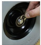
2. Remove both C-clips from the axle using needle nose pliers. Slide the wheels onto the axle. Use needle nose pliers to secure wheels with the C-clips.
