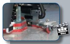
The swinging squeegee (on disc models) is uniquely designed for 100% water pick up, even in turns
