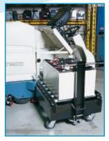
Roll-out battery package extends run-time and is easily changed in less than 5 minutes.
