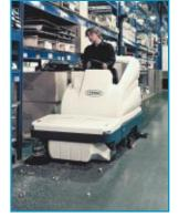
The optional sweeper attachment allows the 7200 to sweep and scrub in one pass.
