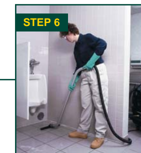
STEP 6 Recover dirty water with the floor squeegee tool and separate recovery hose.
