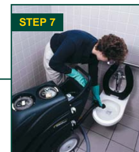
STEP 7 Empty recovered water into toilet, mop, sink or floor drain using the drain hose.
