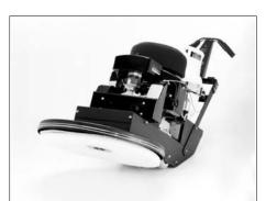
**Pad Change Position** In the pad change position, the Warhorse 27 rests on the two smaller wheels and two rubber feet at the rear of the buffer.
