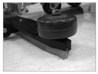
The unique breakaway squeegee assembly on the Wrangler 2016 keeps the machine working when others must be taken off the job to be repaired. If the assembly is inadvertently caught on a fixture or doorway, it releases from the holding bracket at the rear of the machine without bending or breaking. The assembly can be easily re-installed by simply hand tightening two control knobs.
