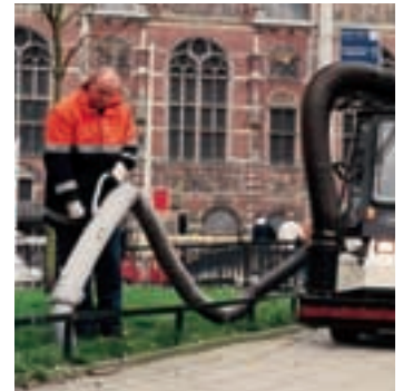
An optional vacuum wand lets operators clean hard-to-reach places.
