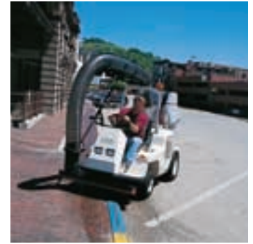
A four-wheel stance provides greater stability, lessens the risk of tip-overs, and gives a smooth ride.
