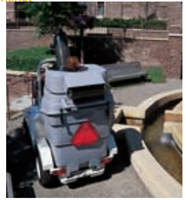
Large capacity hopper means much longer operation before debris dumping.
