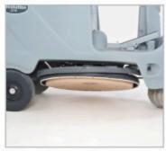
Mid-mounted, burnishing head tilts up for access to change burnishing pads quickly and easily
