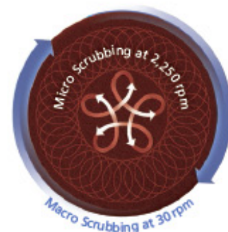
REV model only – Patent-pending REV™ random orbital scrubbing technology with high-speed, ¼-inch micro scrubbing and rotational, low-speed macro scrubbing attacks dirt from multiple directions for superior cleaning effectiveness.
