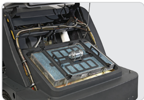
Patent pending Liberator™ Variable Frequency Filter Shaker System removes dust more effectively from the panel filter, resulting in better air flow and dust control.
