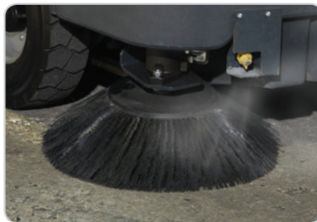
DustGuard™ suppresses airborne fugitive dust where most dust is generated – at the side brooms
