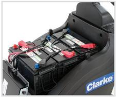
**Batteries** Choose between wet cell or service-free AGM batteries.
