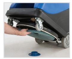
**Pad Changes** Pad changes are easier with the tip back design of the Ultra Speed<sup>®</sup> 20.
