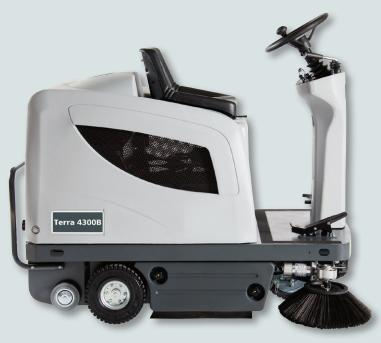
The Terra 4300 sweeper features an aluminum pre-filter panel that traps light bulky debris in the hopper. The pre-filter prevents clogging while offering optimum dust control. And its electric filter shaker provides excellent filter clean-back. The large four-sided steel manual dump debris hopper allows for maximum debris capacity without overflow. The hopper is easy to remove, while the dolly wheels provide a quick method to transport and empty dirt and large debris.
