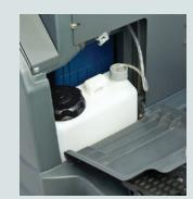
Easy access to onboard detergent dispensing system bottle on EcoFlex™ System.
