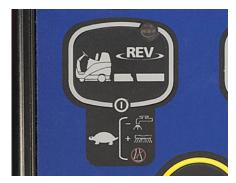
$\mathsf{REV}^{\mathsf{IM}}$  Model Only – When in scrub mode, the One-Touch<sup> $\mathsf{IM}$ </sup> REV $^{\mathsf{IM}}$  function activates floor finish removal operation.
