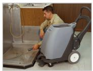
Positioned at the lowest point in the tank, the drain hose provides an alternative draining method.
