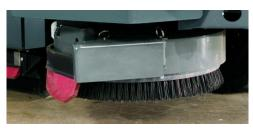
Widen the cleaning path from 40 up to 56 inches / 1,020 to 1,420 mm
