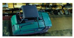
Protect the operator and machine Ensure safety in severe environments with an overhead guard.
