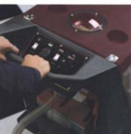
Simply raise the solution/recovery tank for easy access to deep cycle batteries and moisture protected components.
