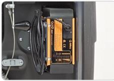
Warrior^  $AXP^{\rm TM}$  scrubber includes a standard onboard battery charger for wet or gel battery packages.
