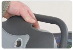
Soft-Touch<sup>™</sup> Paddle System prevents finger pinching, provides maximum control, reduces repetitive-stress injuries, and prevents the operator from being pinned between the machine and an obstruction.
