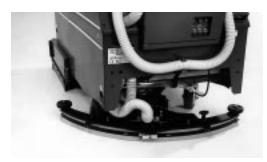
The center pivot squeegee drys better on corners and pivots around obstacles, preventing damage. Leaves floors clean, dry and safe.
