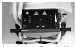
Just twist the grips and go. The easy "twist-of-thewrist" handgrip control doesn't tire the operator. Solution and brushes start and stop automatically. Curtis control gives fully variable speed, both forward and reverse.
