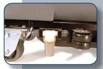
Externally mounted solution filter
