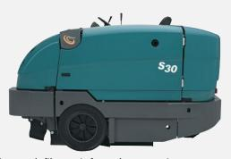
Engineered, fiber-reinforced composite covers are light weight, corrosion resistant, and manufactured with a high-density material. The superior finish makes these covers easy to clean and restorable even if damaged.
