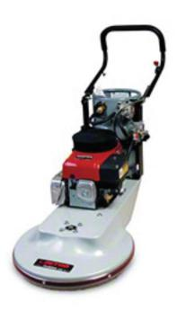
A Honda engine delivers the necessary power to maintain high speed floor finishes in all types of applications.
